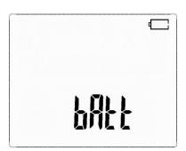
Message **bAtt** indicates that batteries/rechargeable batteries are totally discharged, all measurements are blocked.
