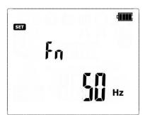
After switching the meter ON, a screen is shown with network frequency settings **Fn**.
