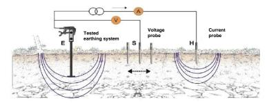
The scheme of measuring the earthing resistance with the 3-pole method is shown above. The figure shows the measurement of earthing resistance  $R_{\text{E}}$ . To perform the measurement, use two auxiliary electrodes:
